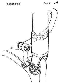
The anti roll bar must be absolutely centered to the car.
