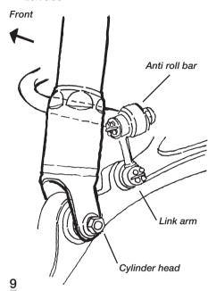
Attach the lower bracket to the wishbone and preload the spring.
